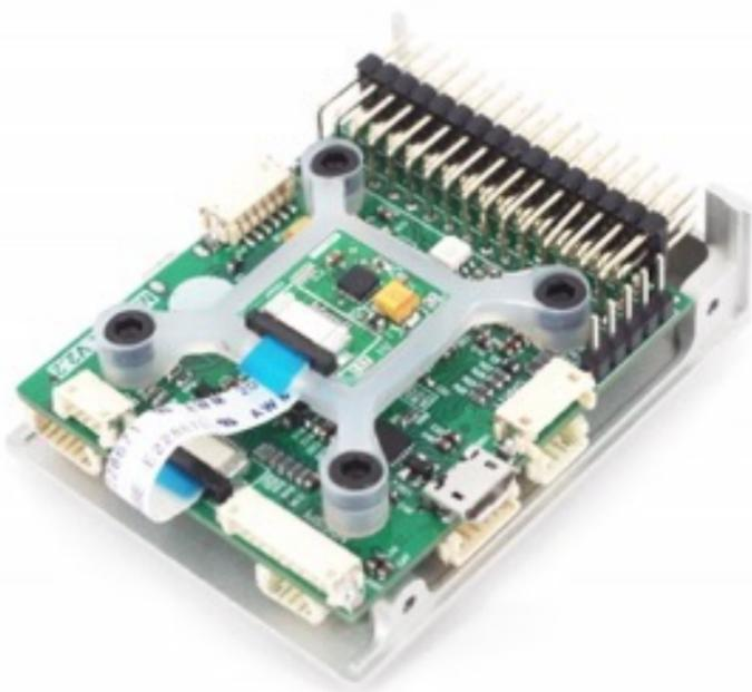
With ingenious design MindPX packs a built-in vibration damping structure into such a compact space.
